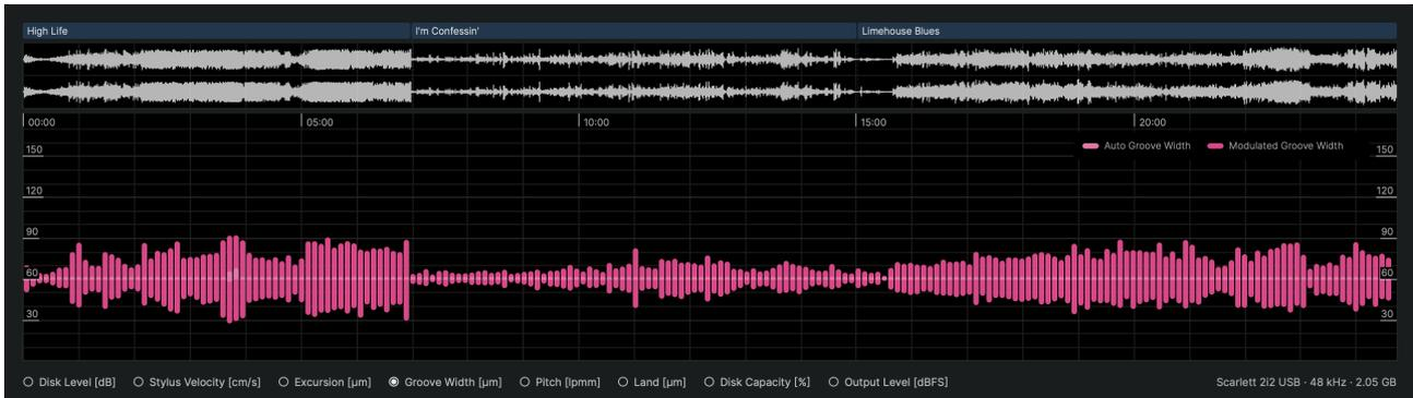
For a purely lateral mono signal, the groove width remains constant at the basic width setting. When stereo content is present, the cutting stylus also moves vertically, which modulates the groove width.
