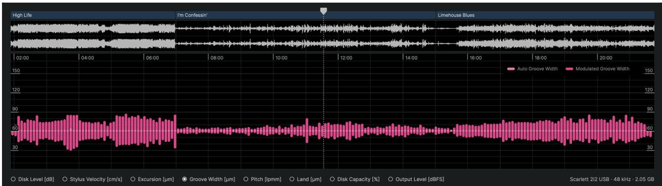
The lower section of the main window presents a waveform of the audio program alongside the results of the groove analysis, arranged on a horizontal timeline.
